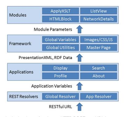
Modules typically obtain data by performing an HTTP POST to a URI that returns an RDF document. That URI can exist anywhere on the internet. If the URI happens to be in Profiles, then the HTTP POST will pass through the REST Resolver and be handled by the Profile application. Thus, the Display application usually calls the Profile application multiple times indirectly via the Modules that it tells the Framework to render.
